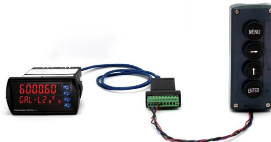
Figure 25. Meter to Control Station Connection
